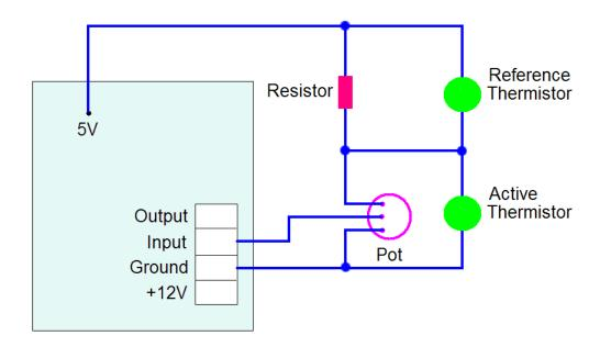
The wiring is carried out as shown here. The 'reference sensor' is placed so that it will be the cooler of the two sensors. When the 'active sensor' is (say) 15 degrees C higher in temp than the reference, the Timer will be switched on. This temp difference can be set by the pot.
