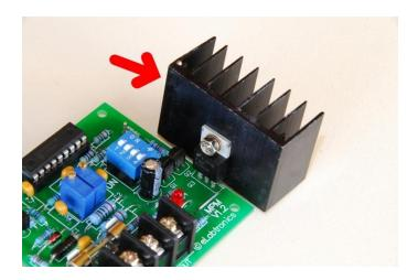
As a general rule of thumb, no heatsink will be needed if you're operating relays, warning globes, LEDs or beepers. If you're operating a pump, a medium sized heatsink like the one pictured will be needed. If you're turning on high powered lights or horns, a large heatsink will be needed.
