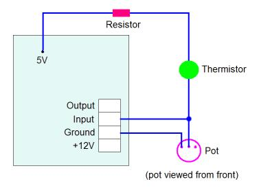
Here is the wiring diagram. Note that for the sake of simplicity, the power and load connections for the Timer are not shown here (or in most of the wiring diagrams in this story).
