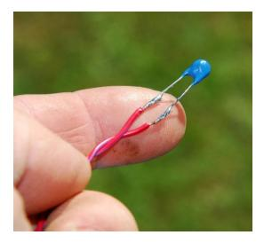
Shorten the leads and then solder two insulted wires to the leads.
