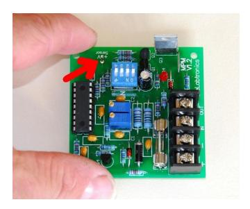
To automatically trigger the Timer on the basis of temperature or light intensity, use is made of a regulated 5V supply sourced from the module. This is available on the pin shown here.
