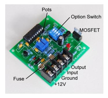
The Timer is based on the eLabtronics Multi-Purpose Module. It has a high current output transistor called a MOSFET, a fuse, four wiring connections, an option switch and two user-adjustable multi-turn pots.
