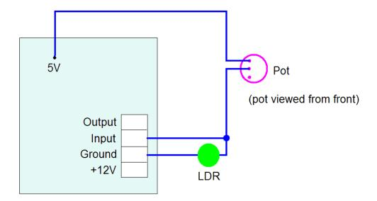
The wiring requires a Light Dependent Resistor (LDR) with a nominal 48 - 140 kilo-ohm response and a 1 meg-ohm pot. Turning the pot clockwise increases the level of darkness needed to trigger the Timer.
