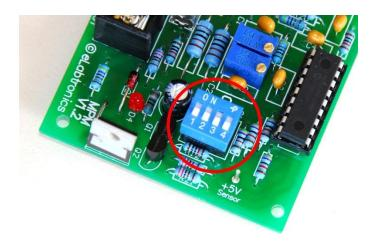
The real smarts in the eLabtronics Universal Timer are in the four-position DIP Option Switch. **Position the board so that the terminal strip is on the right** and then the following switch positions give the listed behaviour.
