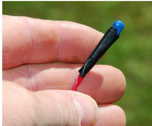
Use insulation tape (when working with relatively low temps) or good quality heatshrink (high temp sensing) to insulate the connections.
